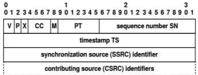
Figure 5: RTP Header
