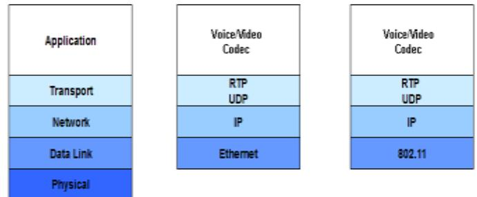
Figure 6: RTP Over different Network Conditions
