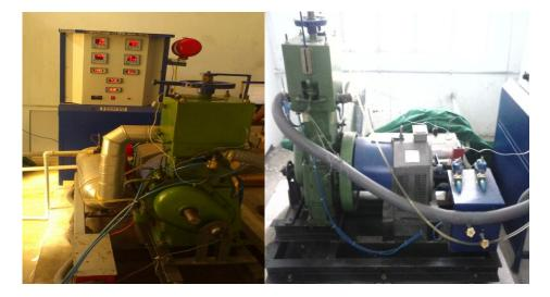
Figure 3.2 Experimental setup of VCR Diesel engine
