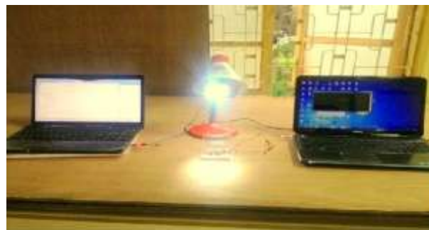
Fig. 1 Prototype of client-server communication using visible light as a medium of communication
