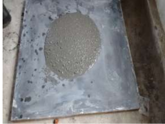
Fig. 1 Slump Spread for SCC with M-Sand
