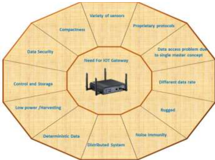
Figure 1: Issues to be handled by Industrial IoT
