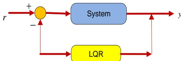
Fig. 4 Linear Quadratic Regulator Structure
