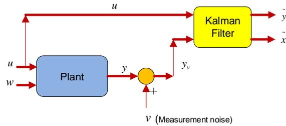
Fig. 5 Block diagram of the Kalman estimator
