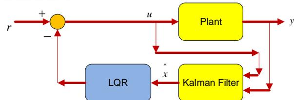
Fig. 6 Block diagram of the LQR control
