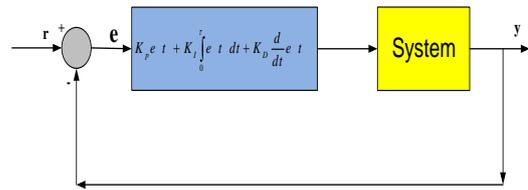
Fig. 3 Block diagram of PID feedback system
