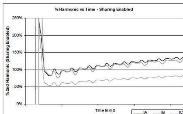
Figure 7 (b) Second Harmonic Content with Sharing Enabled
