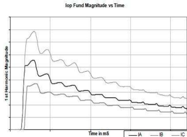
Figure 5 (a): Fundamental Unbalance Current
