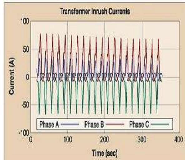
Figure 2: Typical magnetizing inrush current in a power transformer
