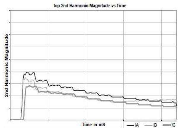
Figure 5 (b): 2nd Harmonic Unbalance Current
