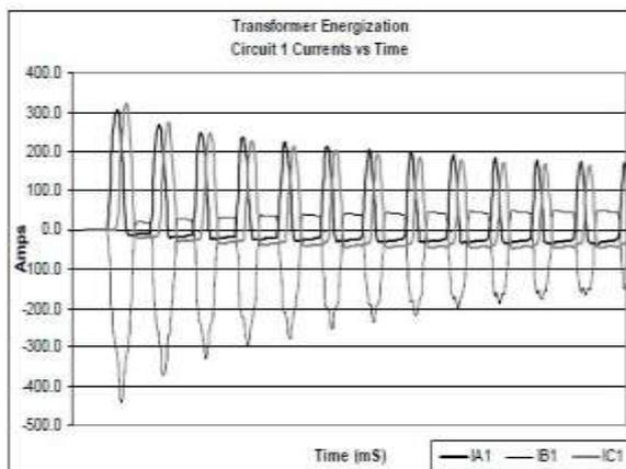
Figure 4: Transformer Inrush Current
