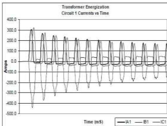
Figure 4: Transformer Inrush Current
