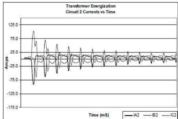
Fig 6: (b) Low Voltage Side
