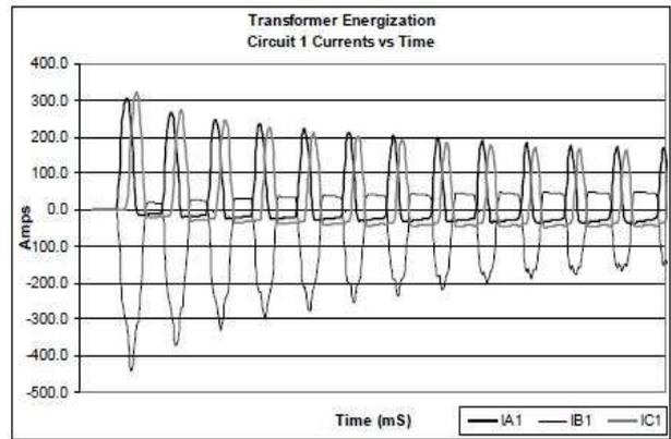
Figure 6: (a) Transformer Inrush Current, High Voltage Side
