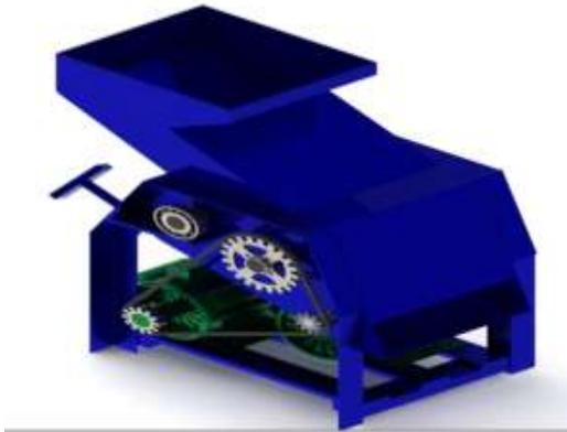
Figure 1: The fabricated double roll crusher.
