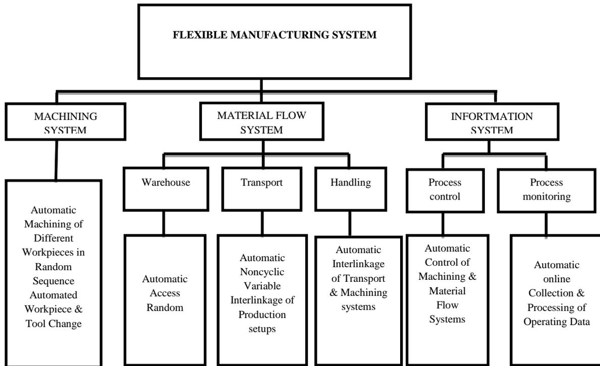
Fig. 1: Components and structure of Flexible Manufacturing System
