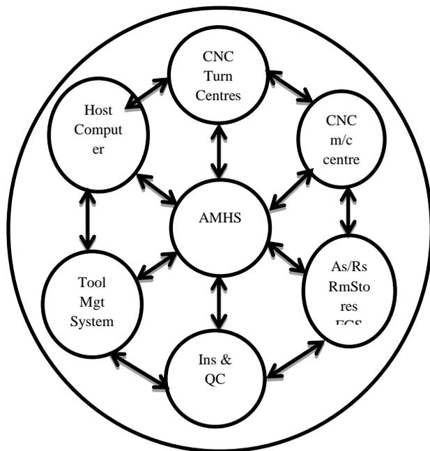
Fig. 2: Components of FMS with interaction and information flow between the sections
