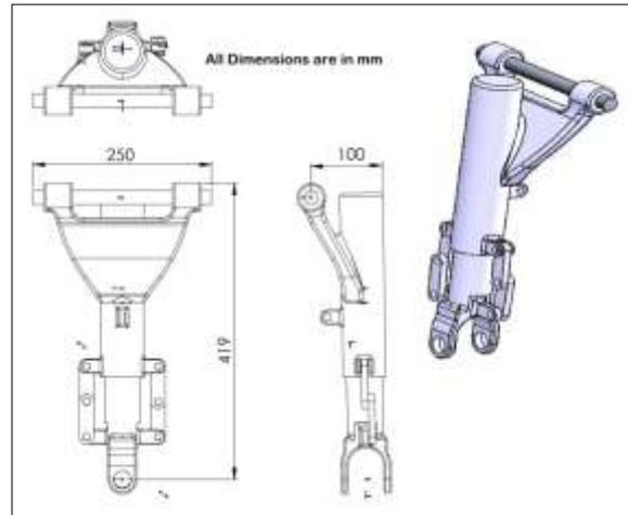
Fig.2 Assembled model of landing gear
