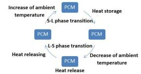
Phase change materials are substances characterized by ability to phase transition at certain temperature range. Scheme of the phase change transition is presented on figure 1. During phase transition there is always heat emission or heat absorption which is called latent heat of fusion. Temperature of transition and amount of latent heat of fusion are distinctive for each material. PCMs are capable to store thermal energy for short or long time.
