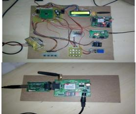
Fig 2: ARM 7 Board (LPC2138) and Receiver unit
