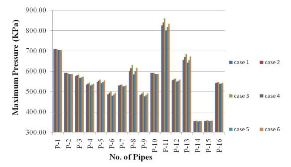
Fig.-3 Maximum pressure in different pipes due to change in pump inertia in Feeder network Phase-1
