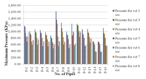
Fig.-5Maximum Pressure in different pipes at different valve closure time in Feeder networkPhase-1
