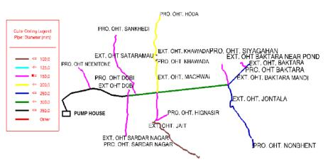
Fig.2 Clear water feeder network phase 2Baneta
