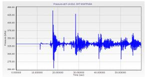
Figure-8 Pressure at pipe P-14 connected to Khatpura for valve closure time 5 sec
