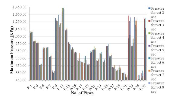
Figure-6 Maximum Pressure in different pipes at different valve closure time in Feeder network Phase-2
