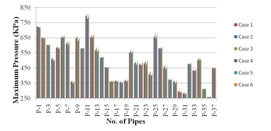
Fig.-4 Maximum pressure in different pipes due to change in pump inertia in Feeder network Phase-2
