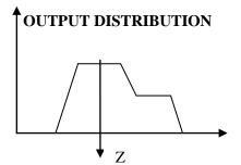
Fig. 4 Defuzzification based on the Mean of maximum
