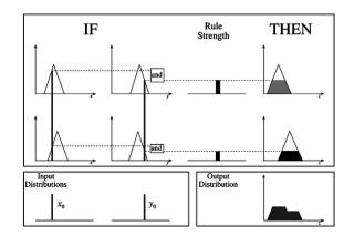
Fig. 2 Diagram showing Mamdani FIS Model with crisp inputs
