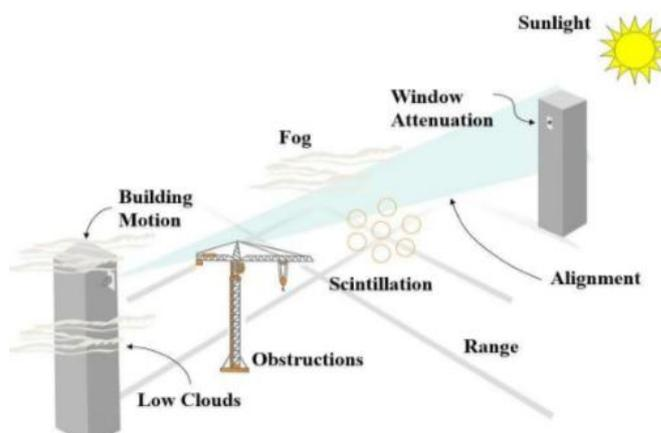
**Figure 2: Challenges in Atmospheric channel [8]**
