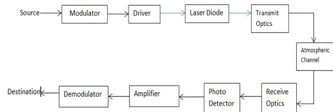
Figure 1: Block diagram of FSO system [3]
