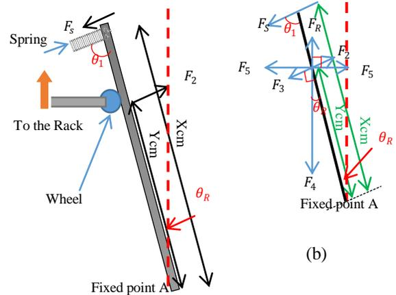
Figure 4. (a) The left deviation plates when rack is moving upwards during the up stroke (b) A sketch showing the force components that act on the deviation plate.
