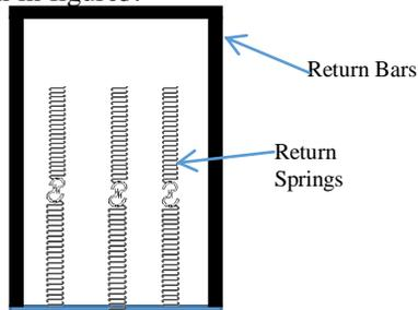
Figure 3. Arrangement of return springs and return-bars.
