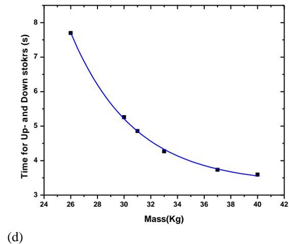
Figure 8.(a) Graph of Total time of rotation against mass; the red curve shows the variation when only the down stroke is utilized, while blue curve shows the variation when both the down and up strokes are utilized to rotate the pinion, (b) graph of power output against mass, (c) graph of RPM against mass, (d) graph of time taken by the rack to make one full stroke against mass.
