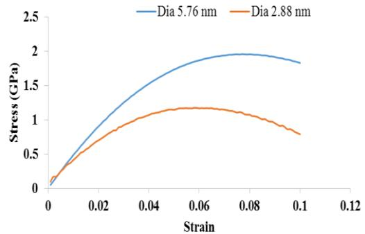
Fig. 3 Stress-strain behaviour of copper nanowire at 0.1K temperature for two different dimensions
