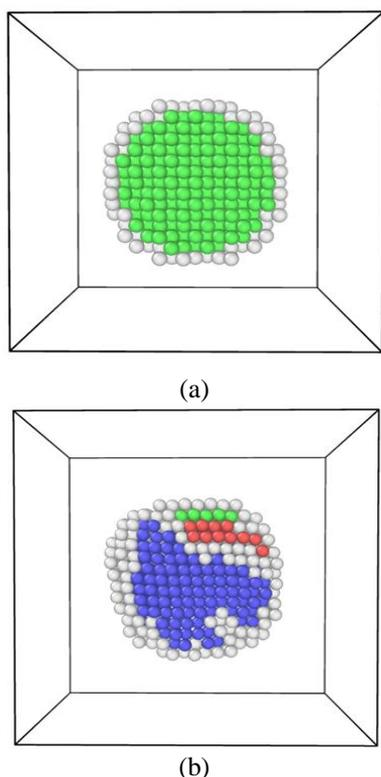
Fig. 9 Change of atomic structures of copper nanowires during compression (a) before compression (b) after 20% strain
