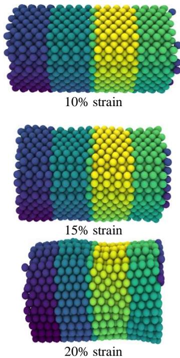
Fig. 5 Nanowires subjected to uniaxial compression at different strains
