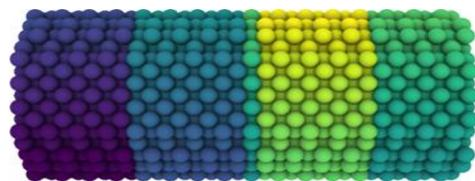
Fig. 4 Equilibrated nanowire model of copper with three twin boundaries
