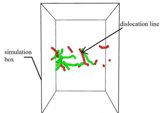
Fig. 7 Dislocations of copper nanowire during compression
