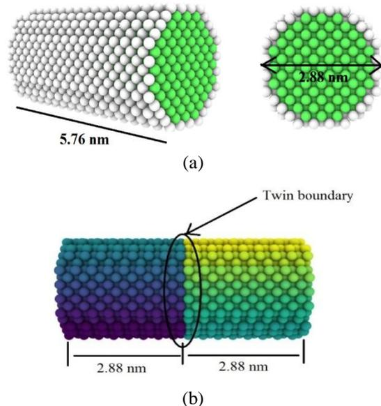
Fig. 1 Nanowire models (a) without twin boundary (b) with coherent twin boundary
