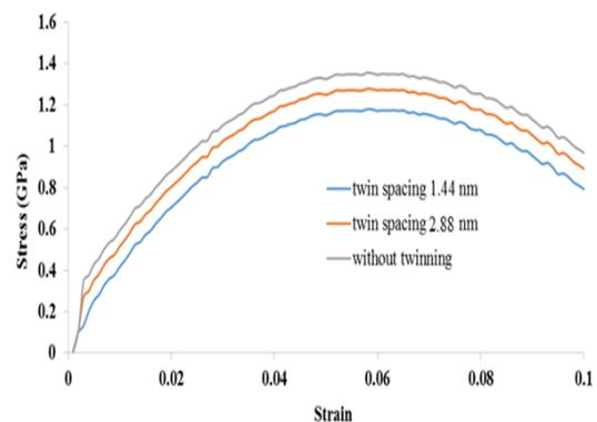
Fig. 8 Comparison of mechanical behaviours of different copper nanowires
