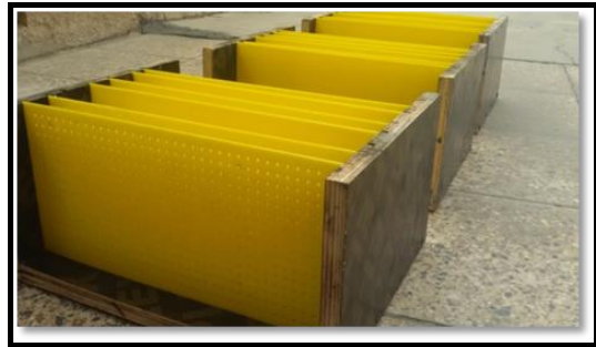
Fig. 1: Details of boards of wood mold
