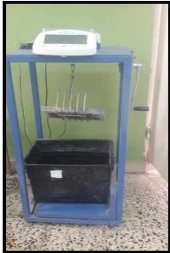
Fig.7: The suspended weight test machine.
