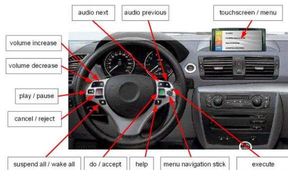
Figure 22: Interactive design using a modern control system.
