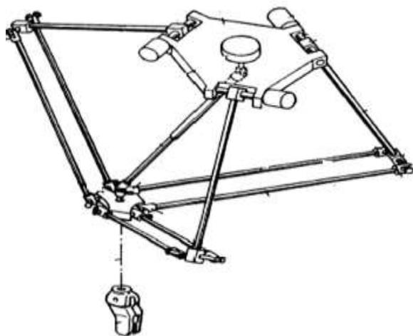
Fig. 2: Mechanical structure of Delta manipulator [10].
