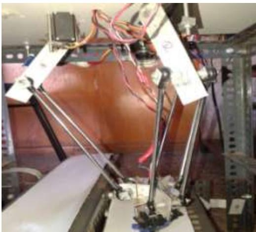
Fig.6: Implemented Mechanical Structure of Delta Robot.
