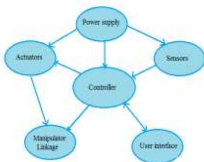
Fig. 3: Components of parallel manipulator
