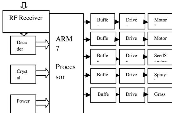
Fig.2. Block diagram multifunctional robotic vehicle system.
