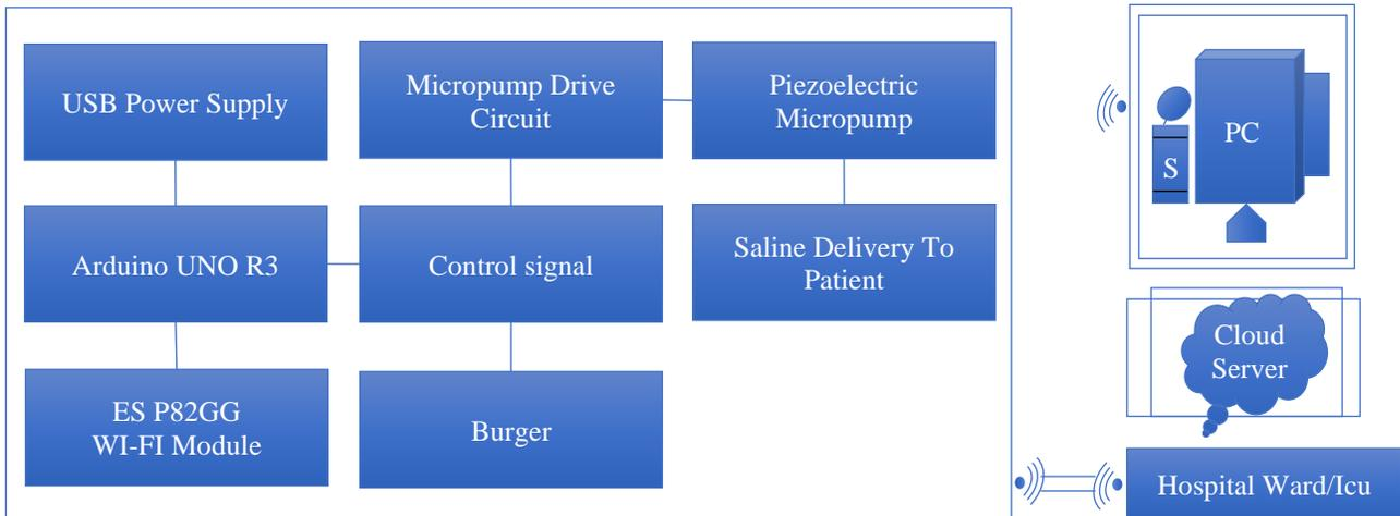
**Fig. 4** Architectural system assembly of the entire project
