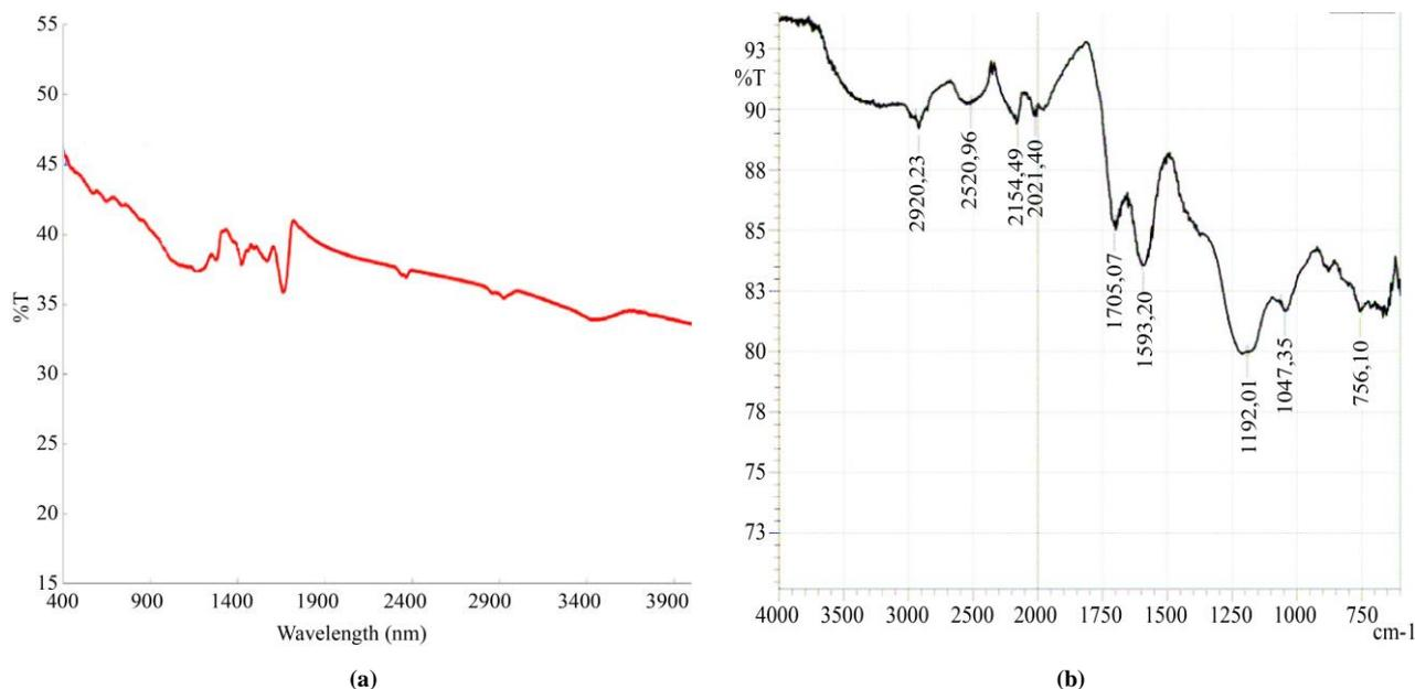
Fig. 4 Infrared spectrum of a) graphite and b) graphene oxide
