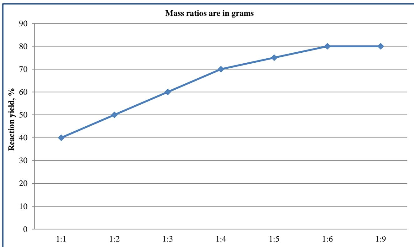
**Fig. 1 The effect of mass ratios of starting materials on the reaction yield during the production of graphene oxide**
