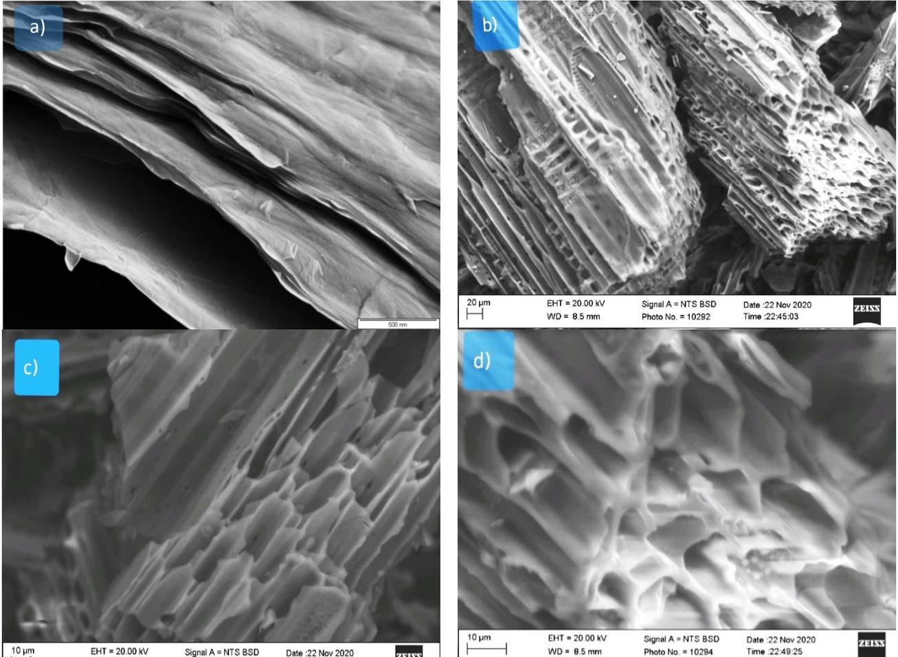
Fig. 5 SEM images of (a) graphite and (b, c, d) graphene oxides
