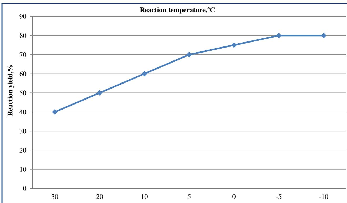
Fig. 3 Effect of temperature on the reaction yield during the production of graphene oxide
