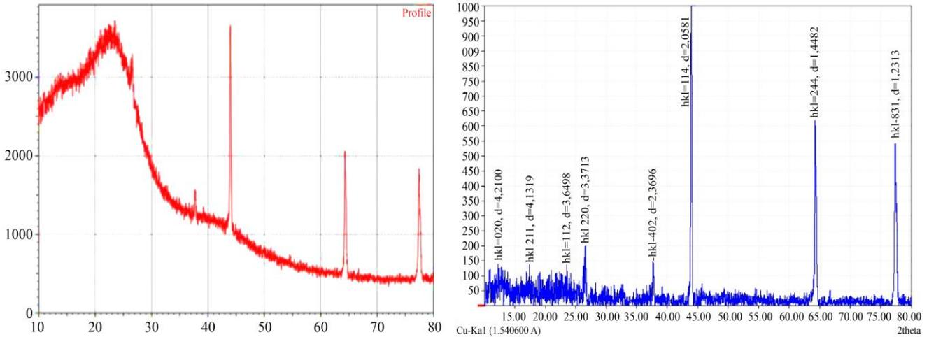
**Fig. 7 An X-ray phase analysis study of synthesized graphene oxide.**
