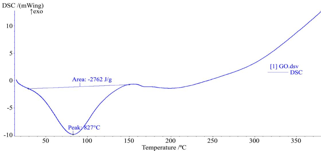
Fig. 6 Thermogram of graphene oxide in a differential scanning calorimeter
