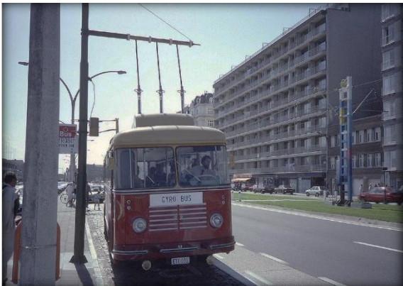
Fig. 2 Flywheel powered Gyro Bus [35]
