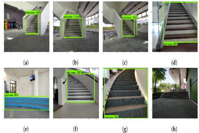
Fig. 13 Staircase detection and localization performance across diverse indoor and Semi-Indoor environments
