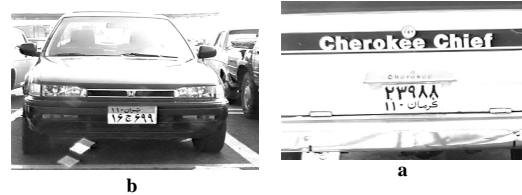
Figure (5): images in which location of the plate can not be recognized by the multiple interlacing method
