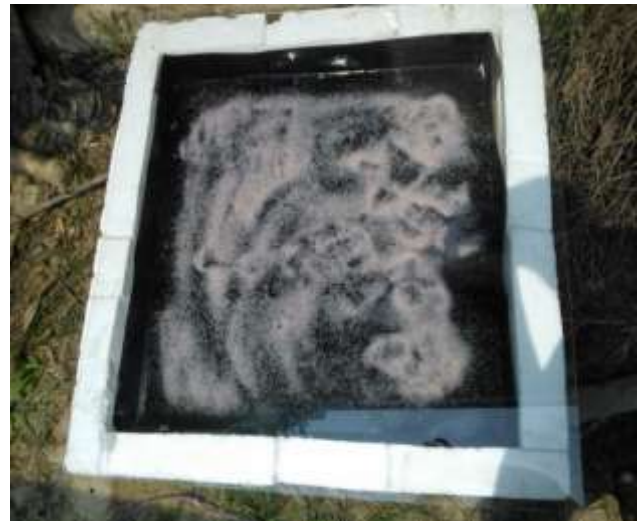
Fig. 10 Solar heater regenerating silica gel
