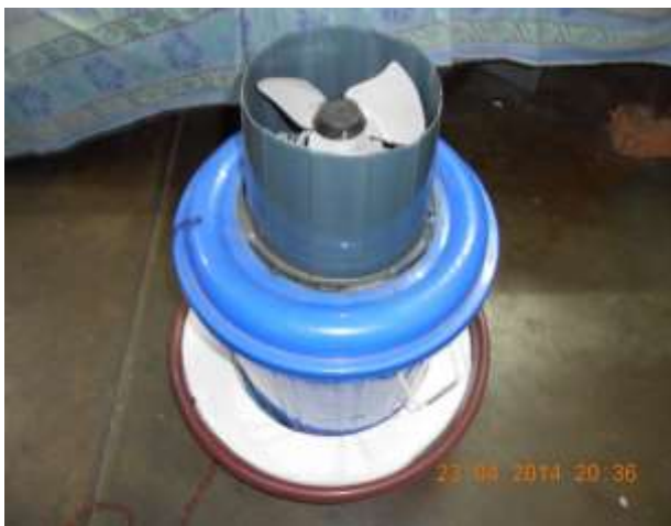
Fig 9: Third model of sweat evaporative fridge
