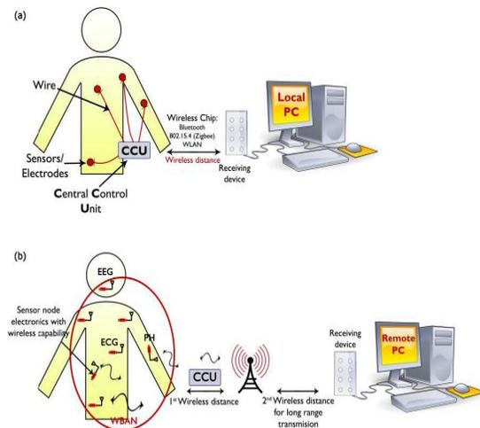
**Figure 1.** A typical WSN system for detecting and transmitting signals from a human body: (a) current application of healthcare sensor network and (b) future application of healthcare sensor network targeted by wireless body area network.
