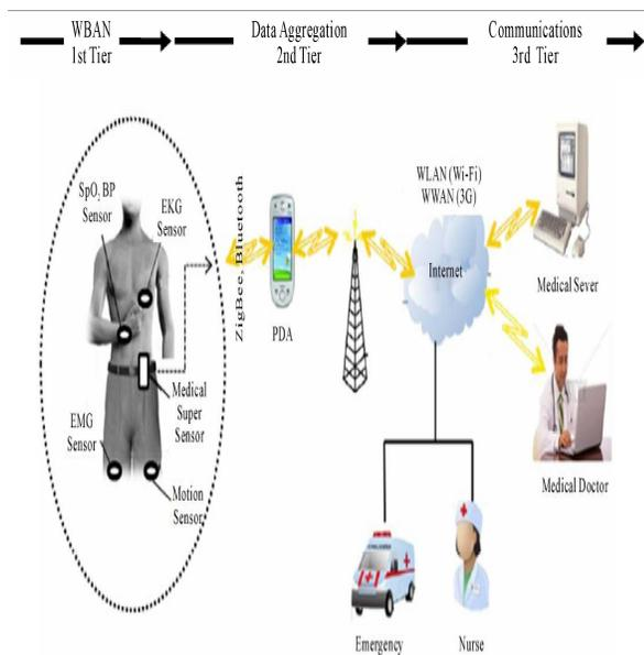
**Figure 3 Architecture of wearable sensors for remote healthcare monitoring system**
