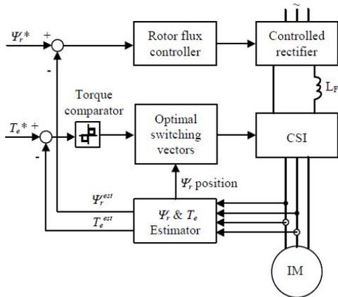
Fig. 1 Conventional DTC CSI-fed IM drive
