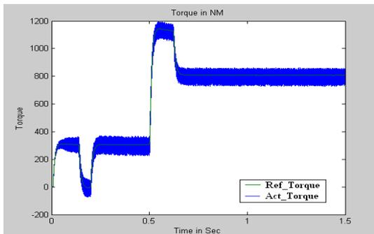
Fig. 4 (c) Torque for Conventional DTC
