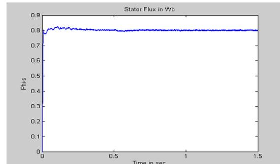
Fig. 5 (b) Stator Flux for Proposed DTC
