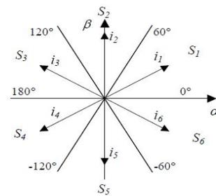
Fig. 2 Sectors in  $\alpha - \beta$  plane where rotor flux resides
