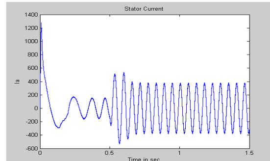
Fig. 5 (a) Stator current for Proposed DTC
