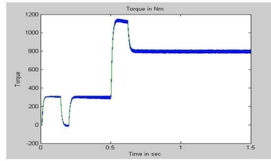
Fig. 5 (c) Torque for Proposed DTC
