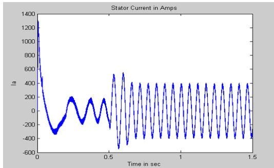
Fig. 4 (a) Stator current for Conventional DTC
