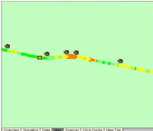
Figure 13 Screenshot depicts drive testing result in dedicated mode on TEMS software. The dark green patches depict a strong received signal. The hand symbol represents handover taking place.
