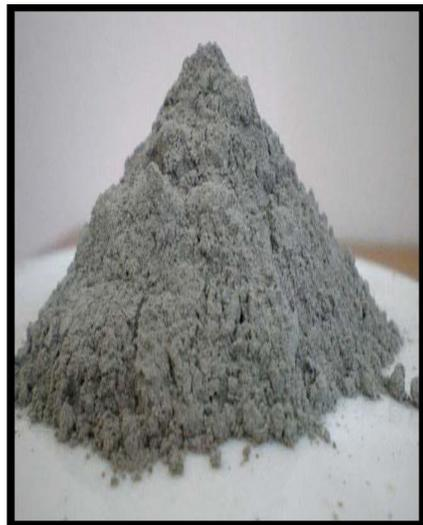
FIGURE 2: Fly ash (Class F)
