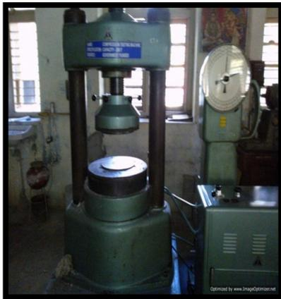
FIGURE: - 6 Compression strength test for Brick
