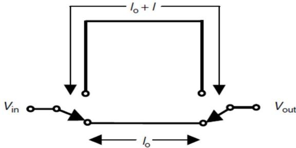
Figure 1. Schematic representation of MEMS switch (PIN diode) as a switched line phase shifter.
