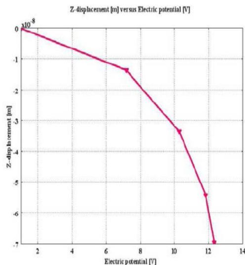
Figure 5. Electric potential Vs. Z-displacement.
