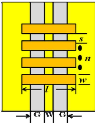
Figure 4. Top view of unit cell structure.
