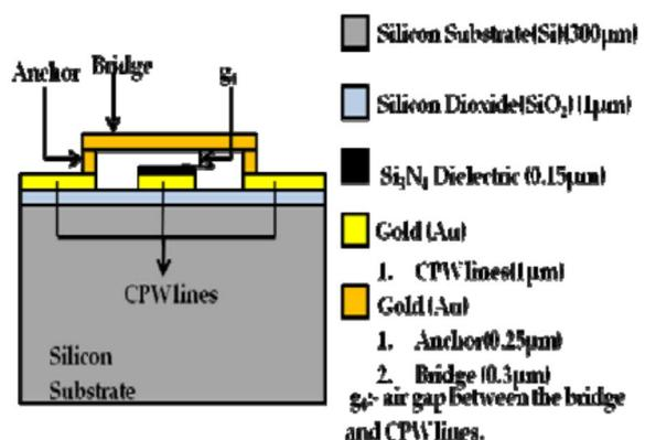
Figure 3. Development of phase shifter unit cell.
