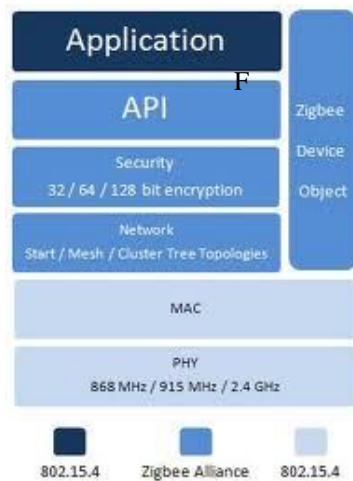
Figure 1 Zigbee layered Architecture
