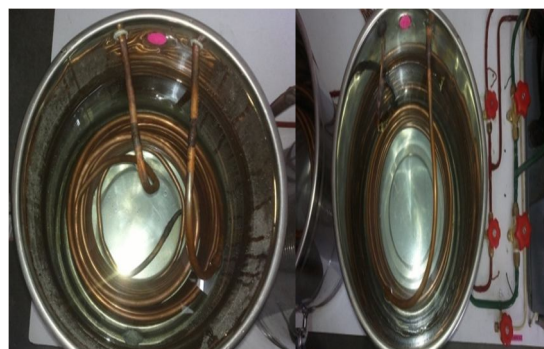
Fig.2.2 Hot water chamber Fig.2.3 Cold water chamber
