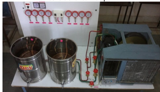
Fig.2.1 Actual set-up of air conditioner cum water dispenser system
