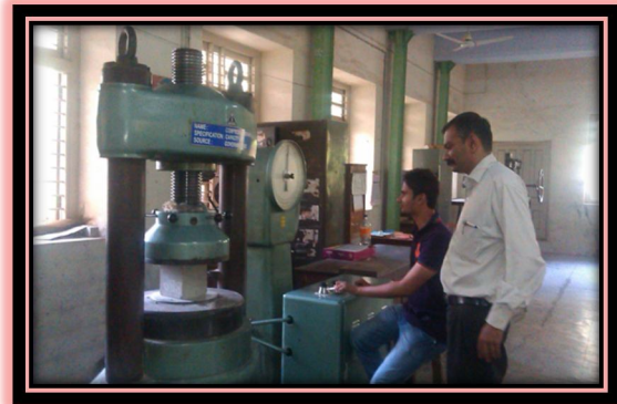
Figure: 5 Setup of Compression Strength Testing Machine with Cube
