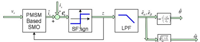
Fig.2 The conventional SMO block diagram with "sign" switching function
