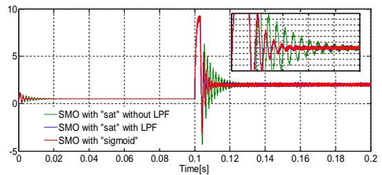
Fig.8 The Electromagnetic Torque control [Nm]
