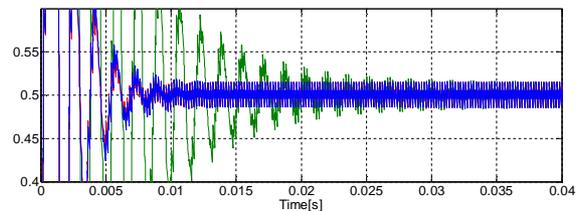
Fig.9 A detailed view of Electromagnetic Torque control for very low speed operation [Nm].
