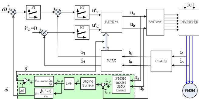
Fig.1 The overall functional scheme of speed and position control of PMSM drive with SMO
