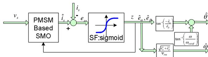
Fig.4 The SMO block diagram with "sigmoid" switching function The state equations of the observer in this case can be represented as:
