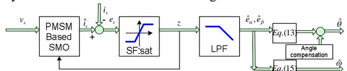
Fig.3 The SMO block diagram with "saturation" switching function
