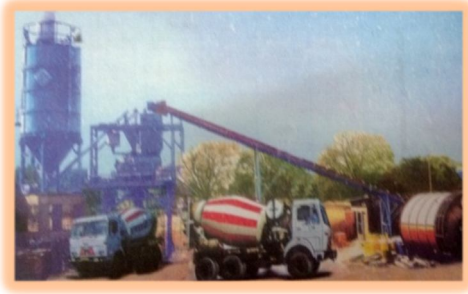
Figure 1 - Modern Ready Mixed Concrete Plant (Source: Concrete Technology Theory and Practice, M.S SHETTY, S.Chand- New Delhi)
