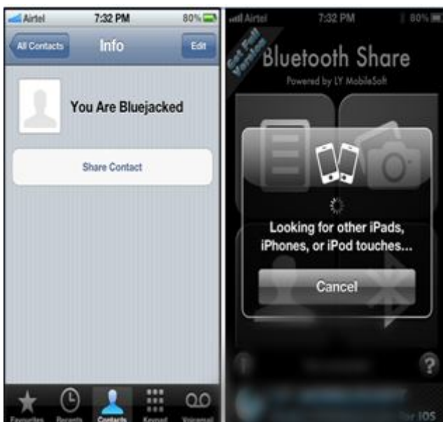
Fig. 6 Contact with name field 'You Are Bluejacked' has been created. Choosing 'Share Contact' -> 'Via Bluetooth' -> message will transmit to victim's mobile
