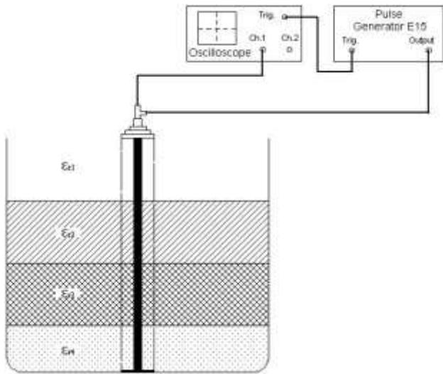
Fig. 4 The adopted arrangement setup used for simultaneous measurement of both liquid level and permittivity in multi-level liquid tank.
