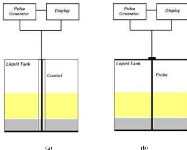
Fig. 3 Measurement setup for; (a) Low viscosity liquids using a coaxial cable sensor, and (b) High viscosity liquids using TDR probe.
