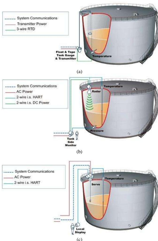
Fig. 1 Different commercial tank gauging systems; (a) float & tape system, (b) radar system, and (c) servo system. [1]
