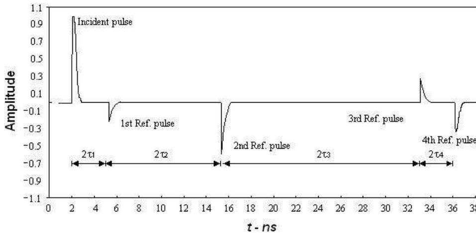
Fig. 7 The simulated incident and computed first, second, third and fourth reflected pulses.
