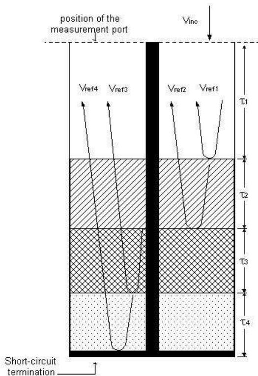
Fig. 5 Liquids are held in a perforated short-circuited coaxial transmission line. The time histories of the incident and reflection from each interface are recorded at a location in the measurement port.
