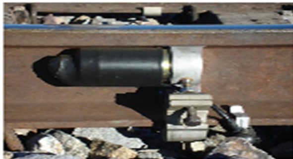
Fig. 3 Ultrasonic based Rail Detection System
