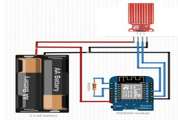
Figure 6. iMHS Circuit Board
