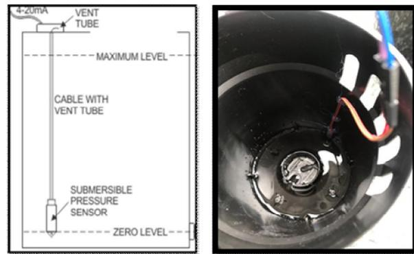
Figure 7. Installation of water level sensor in MHS
