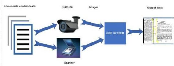
Figure 1: The OCR General Structural [6]
