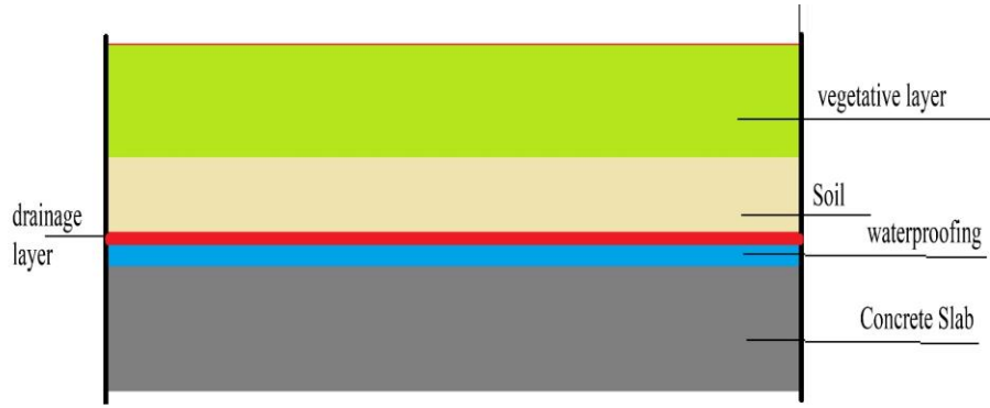
Fig. 1 Diagram of the green roof composition
