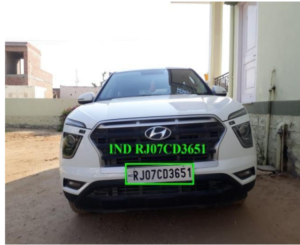
Fig. 18 Final image after extracting vehicle number using OCR technology (Samantaray M 2022)
