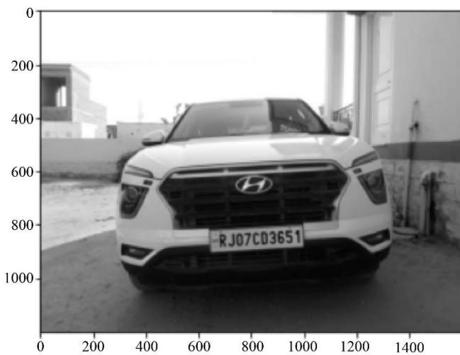
Fig. 14 Image converted to a black and white image to improve the efficiency of the Canny algorithm (Sekehravani E. 2020) for edge detection.
