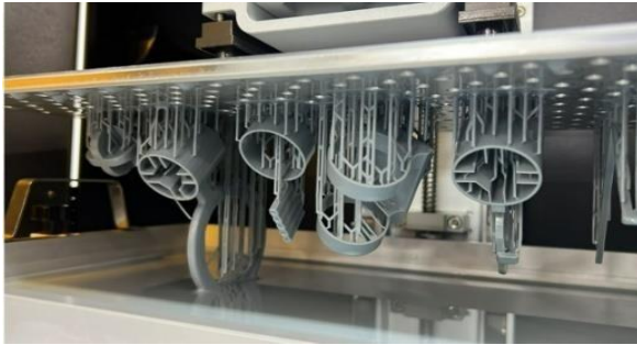
Fig. 9 Fabrication of parts using SLA printer
