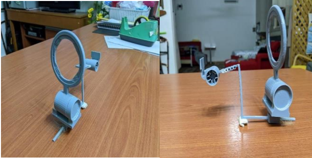
Fig. 14 (a) Fabricated design using SLA printing, and (b) Prototype using all Resin material.
