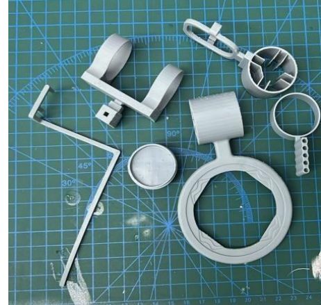
Fig. 12 Drying parts under UV light
