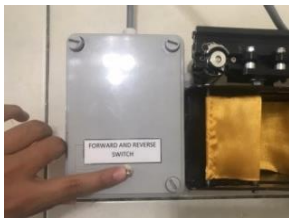
Step 3: Activate the switch to begin the rolling process.
