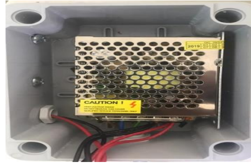
Fig. 6 12V, 5A Power supply unit (QT_12VPSU)
