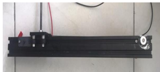
Fig. 8 Steel rail (CYTRON Linear Guide Set)
