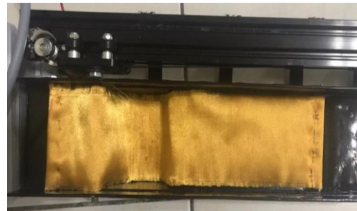
Fig. 7 Cotton fabric as a rotating element
