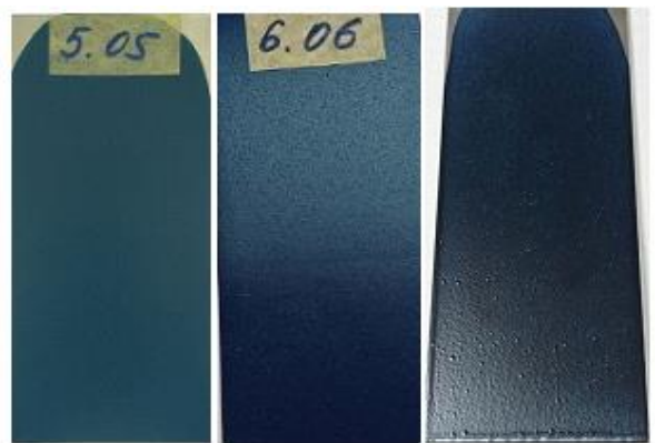
Fig. 9 Alkyd enamel coated on a metal plate (based on new pigments)
