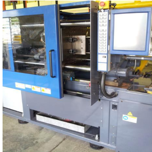
Fig. 1 DEMAG Sumitomo SE100EV series injection moulding machine
