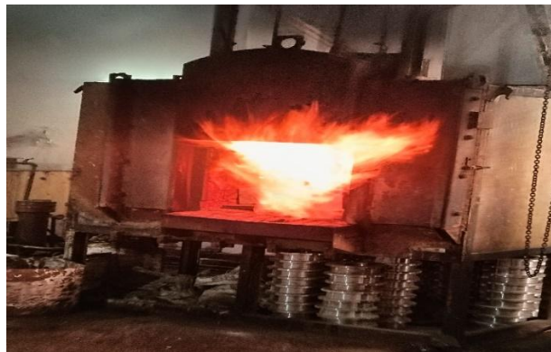
Fig. 2 Specimen exposed to fire in an electric diesel furnace
