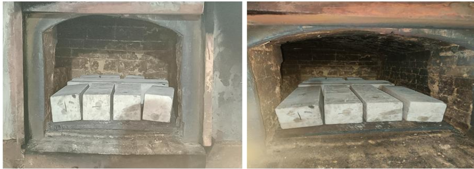
Fig. 1 Placement of casted cubes and beams in diesel furnace
