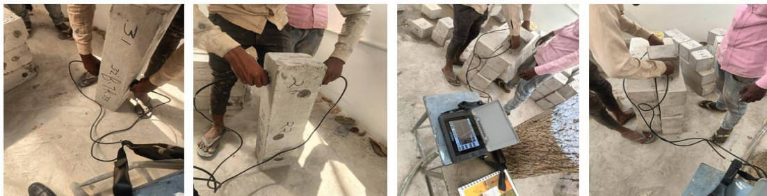
Fig. 4 Ultrasonic Pulse Velocity (UPV) testing of specimen
