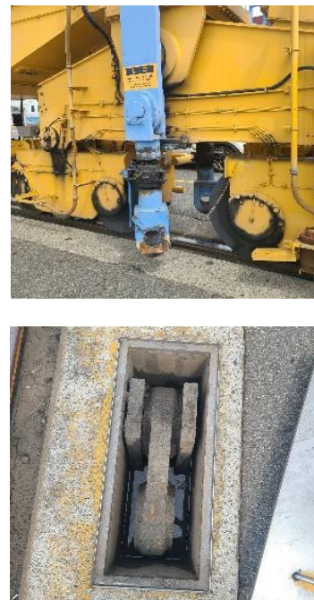
Fig. 3 Example of the installation of a tie down on a port and crane
